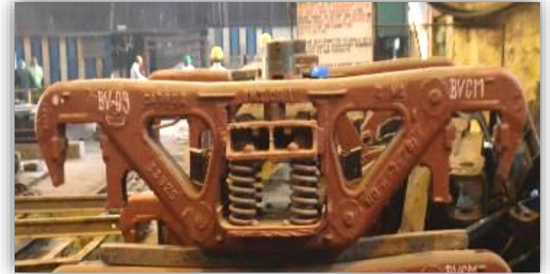
CAST STEEL BOGIE – 22.9T AXLE LOAD
