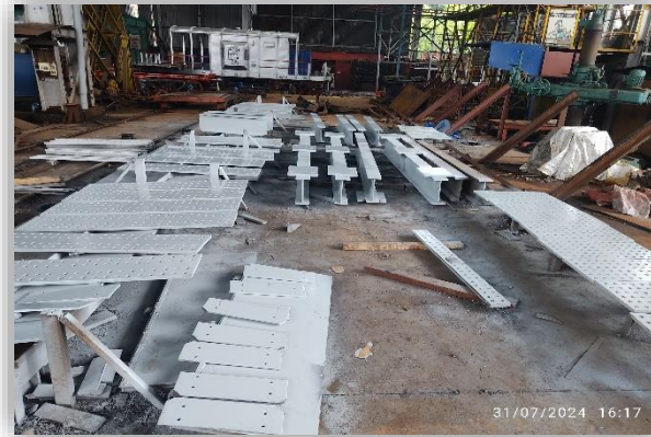
CROSS GIRDER, SPLICE PLATES
